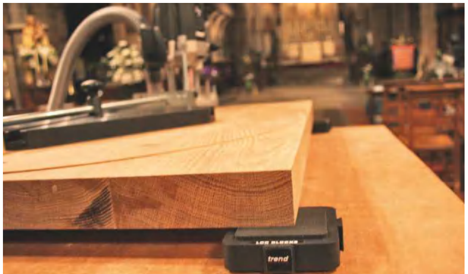
▲ Pic.13 Trend's Loc Block workpiece supports help ensure that everything is firmly held in place
